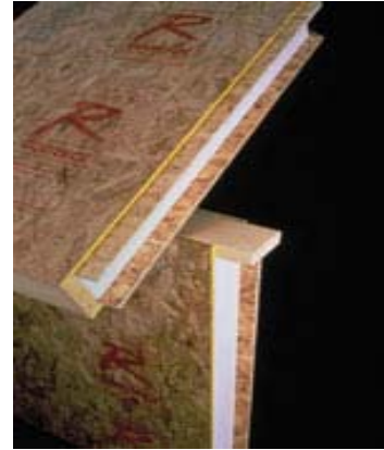
A common SIP is comprised of interior and exterior OSB sheathing with expanded polystyrene core in the middle. CSIPs replace the OSB sheathing with cementitious panel such as Hardieboard. An OSB SIP with splines and top plate installed.
